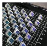
High reflection coating on micro prisms
