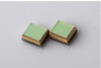
Auto-grade VCSEL module with wide FOV angles for DMS (Driver Monitoring System)
