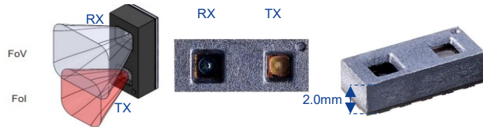
Multi-zone 3D-dToF sensors (~proximity sensors)
