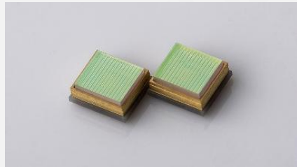
Auto-grade VCSEL modules for DMS (Driver Monitoring System)
