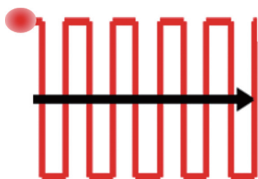
Conventional point laser scanning: Beam must walk through both directions to cover the whole area
